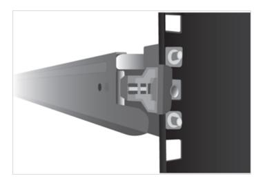
4. Use the attaching screws that came with the mounting hardware to secure the enclosure to the rack.
